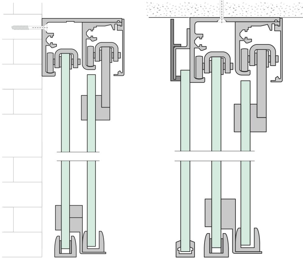
Track fixed to wall or to ceiling, fixed to ceiling with sidelight
